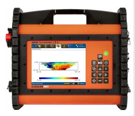
The instrument is a standalone solution featuring built-in measurement channels, high power current transmitter, electrode selector, computer and graphical user interface. Surveying techniques range from 1D to 4D measurements. The robust and rugged aluminum casing meets IEC IP66 classification and allows for use in the harshest of conditions.
